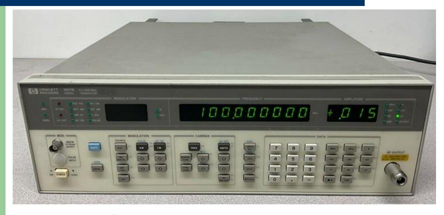
100 kHz to 2.06 GHz, +13 dBm to -143.5 dBm General purpose signal generator Good choice for RX testing if you can justify the price.
