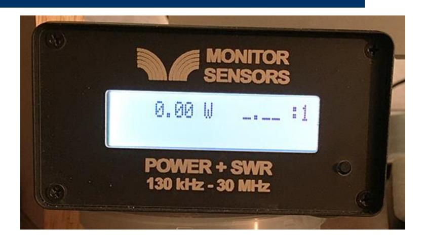
Covers 2200 meters and 630 meters (136 kHz & 472 kHz)
