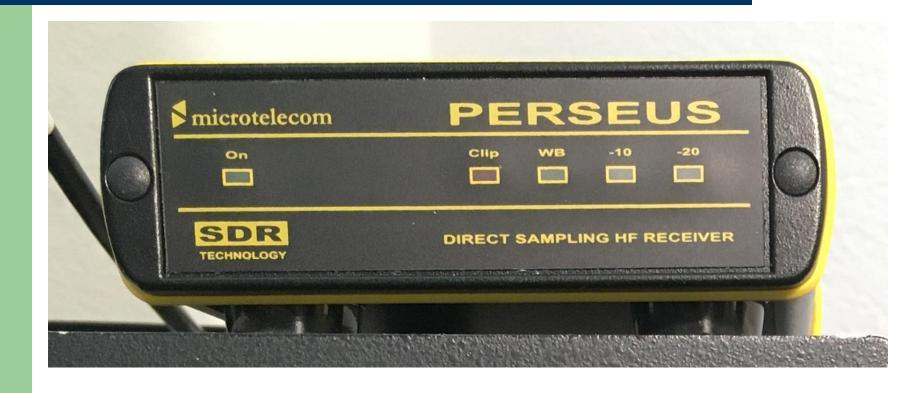
Runs under Windows. Version 4.1a software recommended SDR tunes to 40 MHz. Also measure TX composite noise Have down-converted 2m, 70cm & 23cm signals to 20 meters. Measured the Icom IC-9700 on all bands
